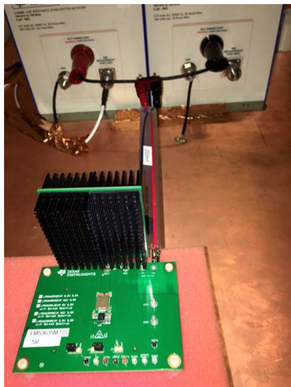
Figure 20. Conducted EMI Setup - Front View
