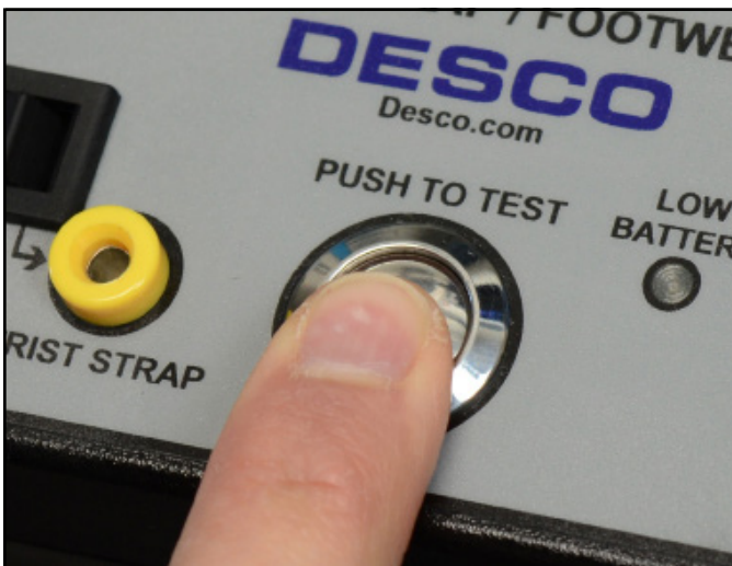
Figure 13. Bridging the pushbutton and its surrounding metal ring when performing a test
