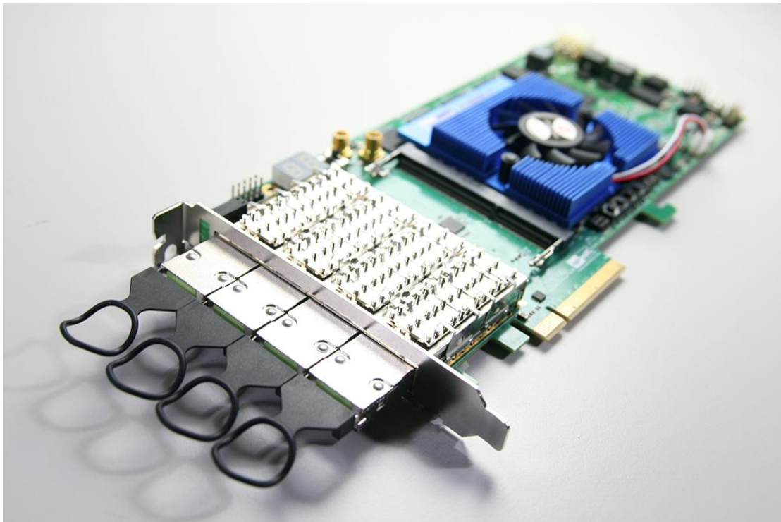
Figure 8-4 Four QSFP+ Loopback Fixtures Installed
