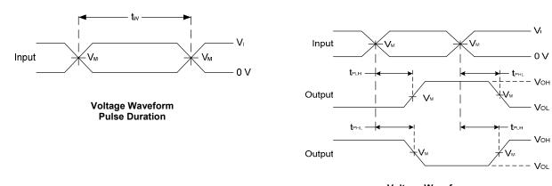
Voltage Waveform Propagation Delay Times Inverting and Non Inverting Outputs
