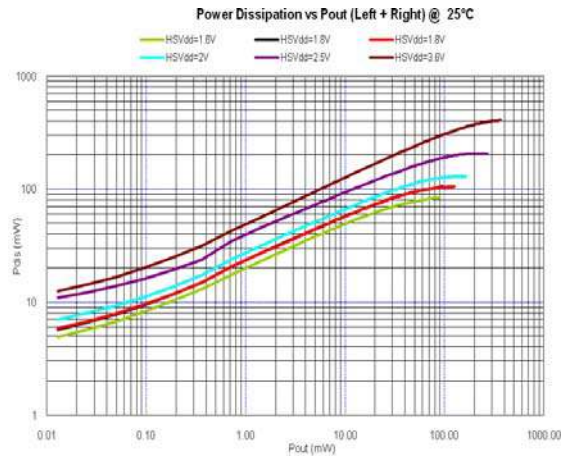
Figure 16. Power Dissipation vs P_{out} with 16\ \Omega Load
