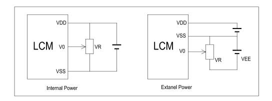
$V_{DD^{\sim}}V_0\text{: LCD Driving voltage}$
