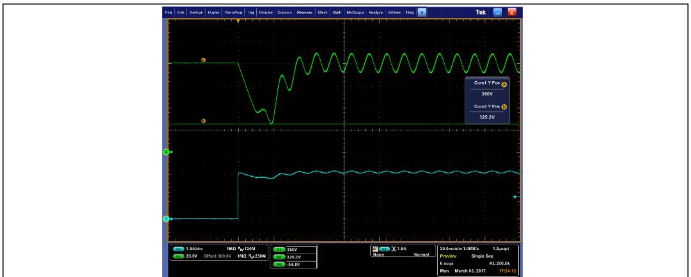
Figure 18 Load step: 0% → 100% at V_{IN} = 115 V AC
