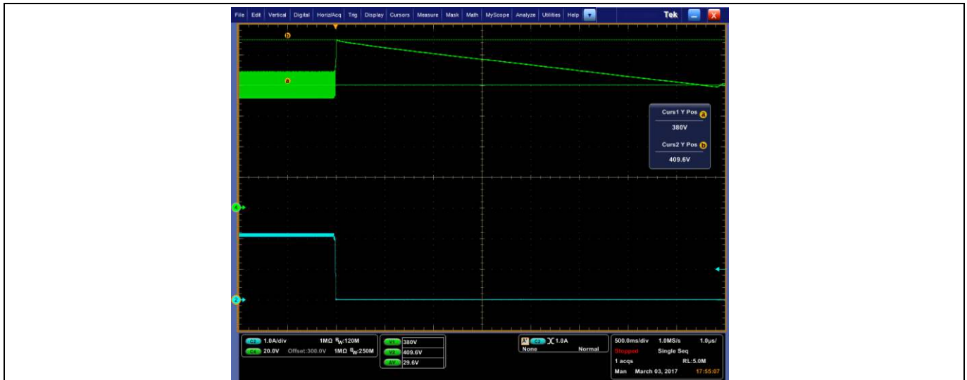
Figure 20 Load step: 100% → 0% at V_{IN} = 115 V AC
