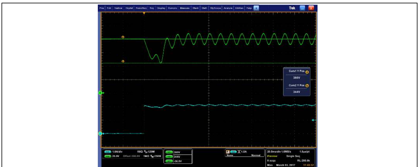
Figure 19 Load step: 0% → 100% at V_{IN} = 230 V AC
