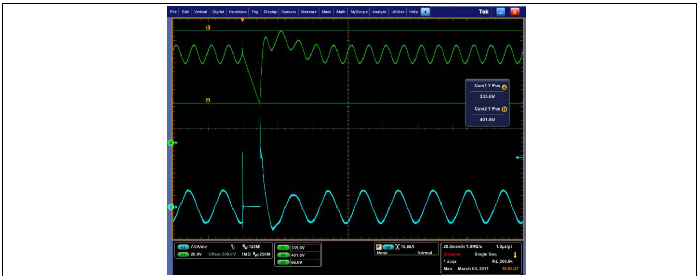
Figure 24 AC line drop out for 10 ms when V_{IN} = 230 V AC at P_{OUT} = 800 W
