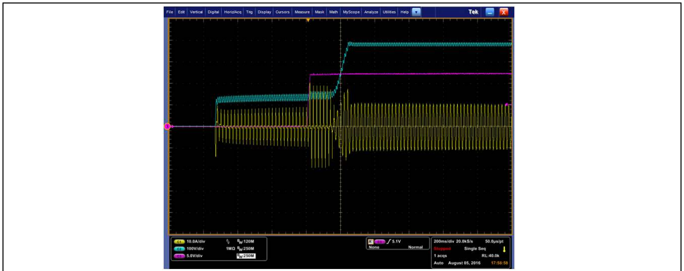
Figure 21 Star-up at V_{IN} = 115 V DC
