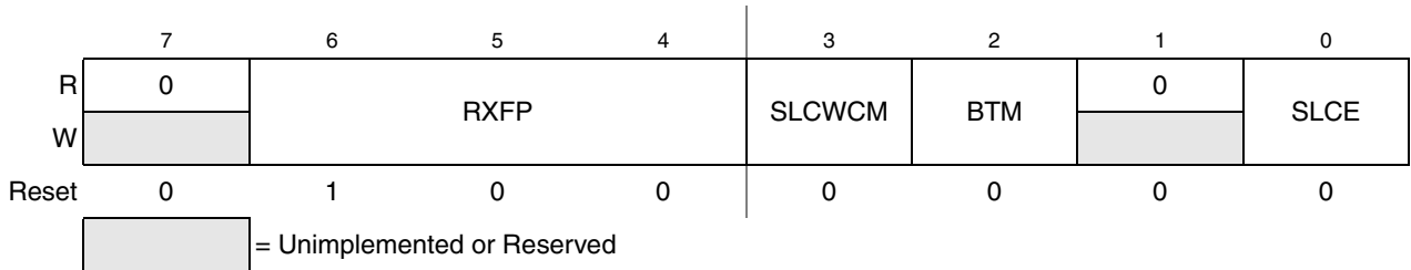
Figure 12-5. SLIC Control Register 2 (SLCC2)
