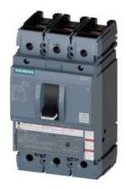
circuit breaker 3VA5 UL frame 250 breaking capacity class H 65kA @ 480 V 3-pole, line protection TM210, FTFM, In=125A overload protection Ir=125A fixed short-circuit protection Ii=10 x In UL489 SB (naval), 50 deg. cel. nut keeper kit on both sides
