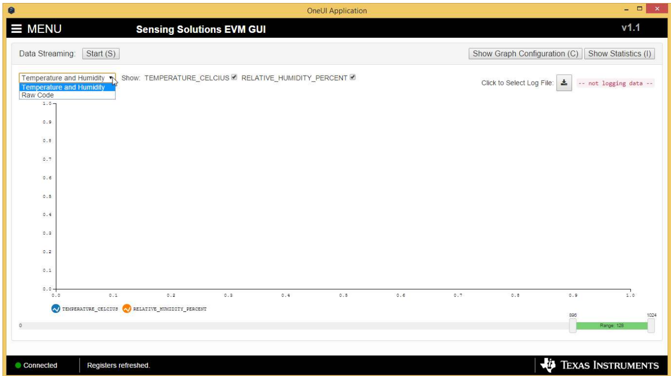
Figure 35. Selecting the Measurement Units for the Data Streaming Graph
