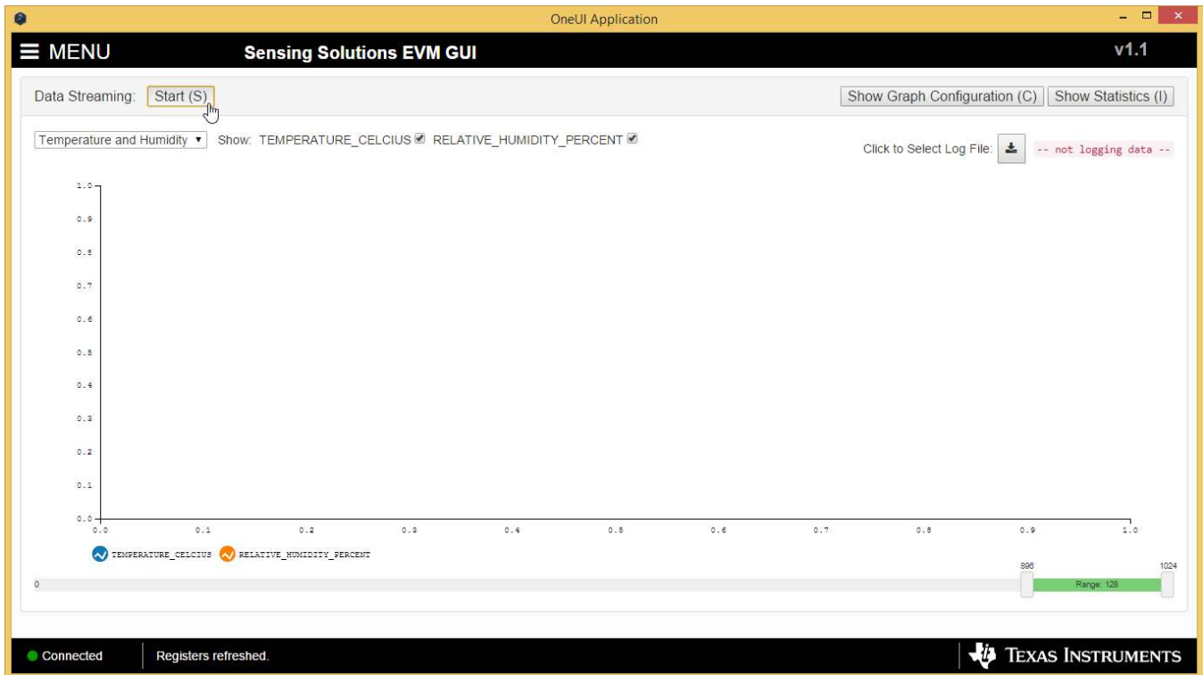
Figure 43. Starting Data Acquisition on Data Streaming Graph
