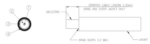
NOTE: JACKET STRIP OD DEFORMED MUST BE THAN LESS Ø2.75mm AFTER CUT OFF.
