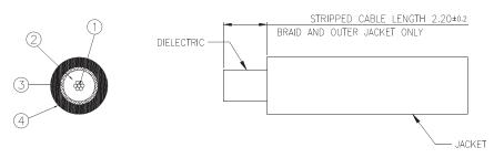
NOTE: JACKET STRIP OD DEFORMED MUST BE THAN LESS Ø3.30mm AFTER CUT OFF.
