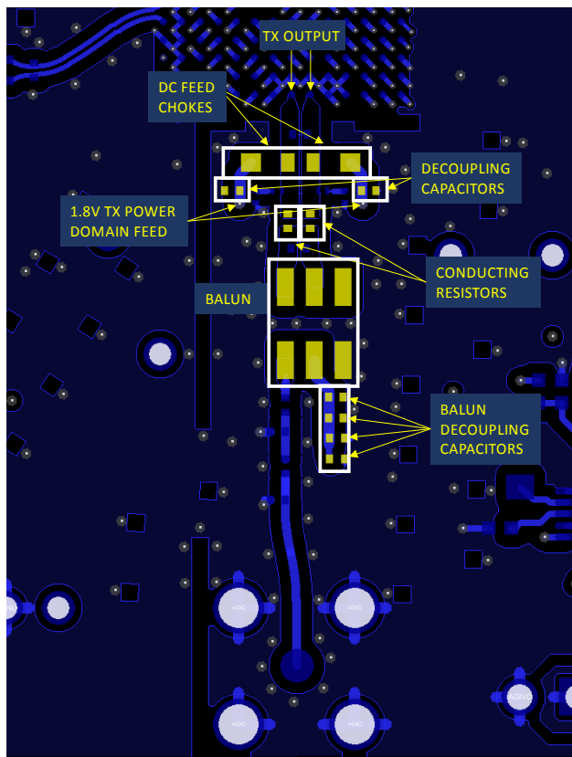
Figure 280. Transmitter DC Chokes and Balun Feed Supply
