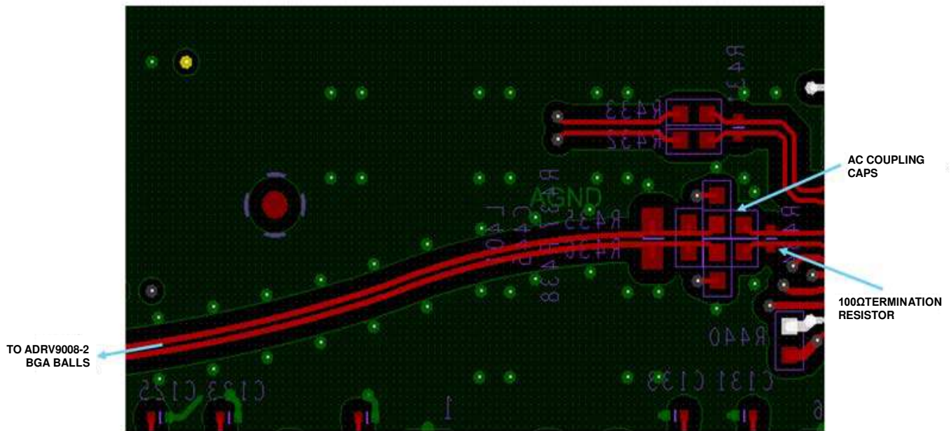
Figure 272. REF_CLK_IN \pm Routing Recommendation
