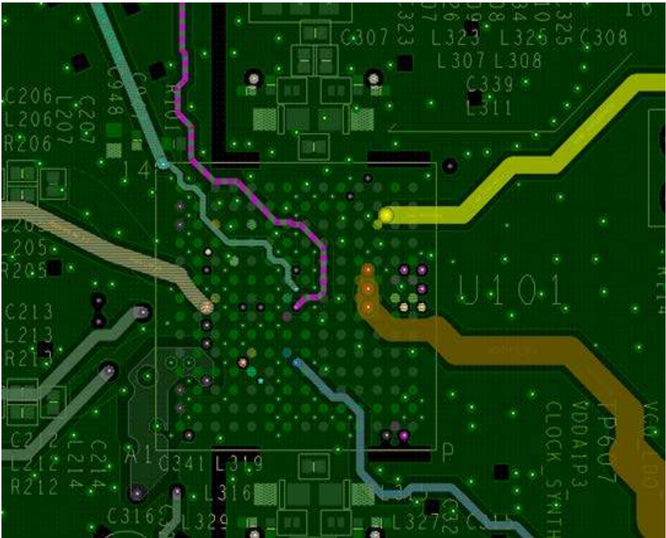
Figure 273. Layout Example of Power Supply Domains Routed with Ground Shielding (Layer 12 to Power)
