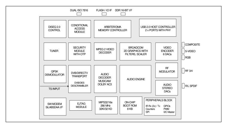
The BCM7312 is Broadcom's third-generation satellite set-top box system on a chip design, but it is the first to fully integrate the DBS Tuner. This is the first truly integrated single chip for DBS applications.
