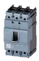
circuit breaker 3VA5 UL frame 125 breaking capacity class H 65kA @ 480 V 3-pole, line protection TM210, FTFM, In=15A overload protection Ir=15A fixed short-circuit protection Ii=20 x In UL489 SB (naval), 50 deg. cel. cable connection on both sides
