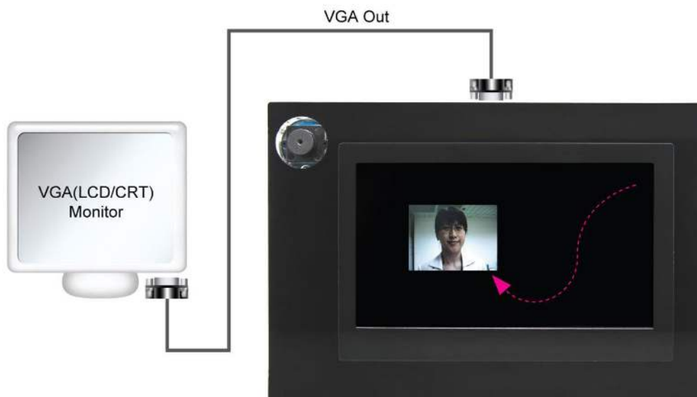
Figure 4-14 Setup for the VIP_Camera demonstration
