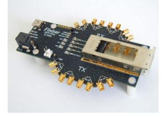
Finisar's FDB-1042 QSFP+ Evaluation Board is designed for testing and evaluating the QSFP+ transceiver and Quadwire<sup>™</sup> Active Optical Cables.
