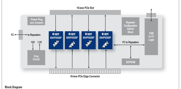
A block diagram of the 89HP0508P Repeater Evaluation Board is shown above. The board design includes four 8-channel 89HP0508P Repeaters implemented in a unidirectional architecture.
