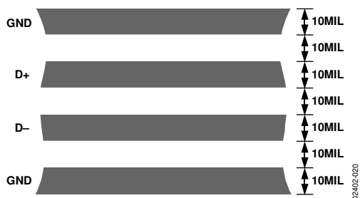
Figure 20. Arrangement of Signal Tracks
