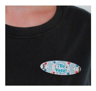
8. Turn it on! One switch is an ON/OFF switch, the other controls blinking vs solid modes for the LEDs. Wear it any way you want!
