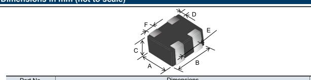
Part No. Dimensions Mass (Weight) (inch size) (mg/pc.) Α В С Ε F EXCX4CE (0202)  $0.50 \pm 0.05$ 0.65 ± 0.05  $0.30 \pm 0.05$ 0.12 ± 0.10  $0.40 \pm 0.10$ 0.15 ± 0.10 0.56
