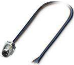
Sensor/actuator flush-type plug, 3-pos., M8, rear/screw mounting, with M8 thread, with 0.5 m TPE litz wire, 4 x 0.25 mm 2
