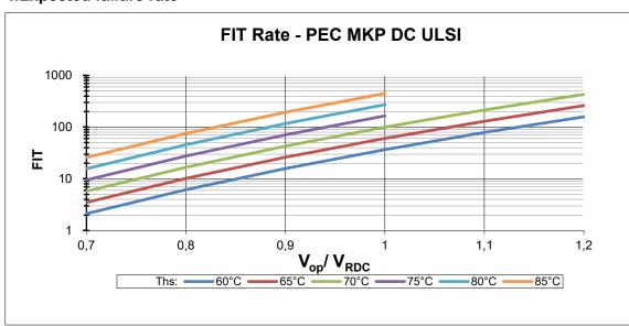
Expected fit rate at different hot spot temperatures (T<sub>hs</sub>) and voltage V<sub>RDC</sub>
