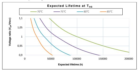
Service life  $t_{LD}$  at different hotspot temperature ( $T_{hs}$ ) and  $V_{OP}$
