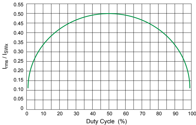
Figure 23. Input capacitor ripple versus duty cycle
