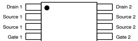
Figure 3. Pinouts for Dual-Die TSSOP
