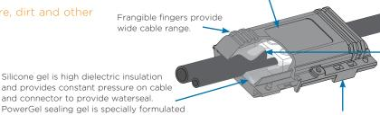
Range-taking mechanical connector made of aluminum. Accepts both copper and aluminum conductors.
