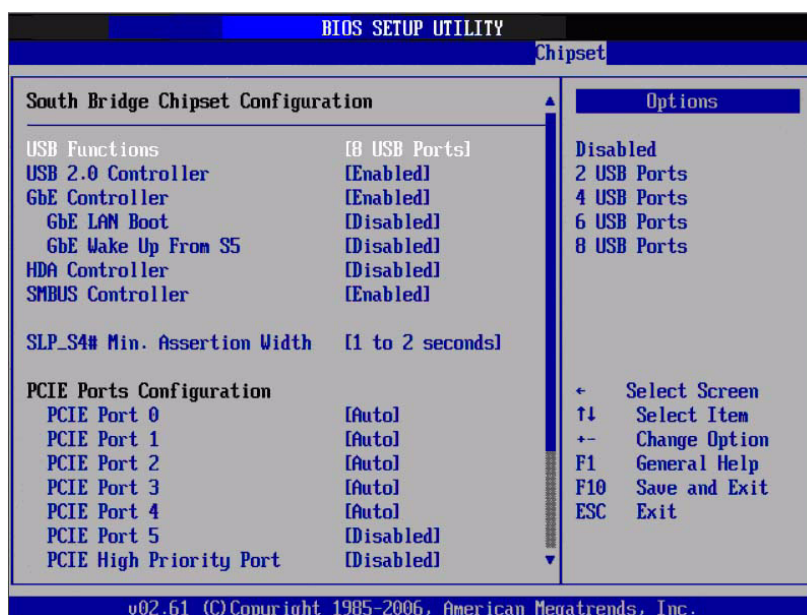
Figure 3.27 South Bridge Configuration
