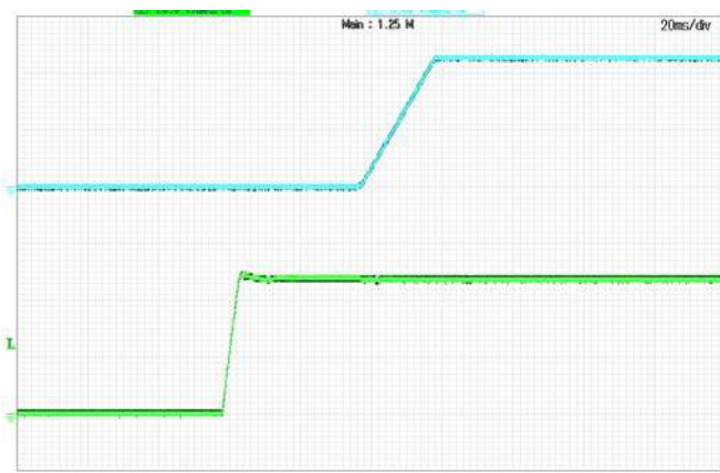
Figure 7: Turn-on transient at full rated load current (20 ms/div). Top Trace: Vout; 5V/div; Bottom Trace: input voltage: 30V/div.
