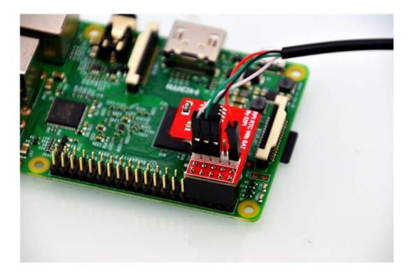
**NOTE**: DO NOT power it again if the Raspberry Pi has been powered, or it will damage the module and Raspberry.
