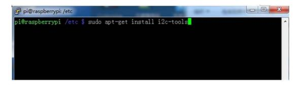
• 8. Input "sudo reboot" to reboot Raspberry Pi; Input "sudo i2cdetect-y1" after a reboot. If everything goes well, the module will be detected normally.
