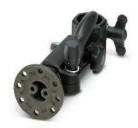
140.5 mm housing attachment, for max. load 10 kg, with ball joint and fastening plate 60 mm, pivotable in  $15^\circ$  increments, for 30 mm wall/profile bracket, material: black glass-fiber reinforced polycarbonate PC, and black anodized aluminum, 342~g
