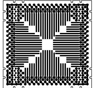
Support up to 84 pins PLCC package IC with 0.05" pitch, 26 pcs. of 0603 package, and some thru hole passive components. 14 ground holes are connected a copper plane on the bottom side.
