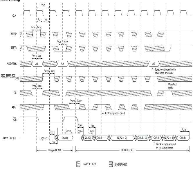
**Note:** 16. On this diagram, when  $\overline{CE}$  is LOW,  $\overline{CE}_1$  is LOW,  $CE_2$  is HIGH and  $\overline{CE}_3$  is LOW. When  $\overline{CE}$  is HIGH,  $\overline{CE}_1$  is HIGH or  $CE_2$  is LOW or  $\overline{CE}_3$  is HIGH.
