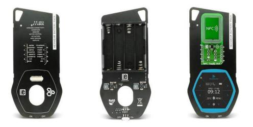
**Hexiwear Battery Pack** will keep your favorite IoT development kit charged. You can add any functionality with the onboard mikroBUS<sup>TM</sup> socket. Add sensors, transceivers, speech recognition modules and more. No more cables and worrying if the battery on it will last the day.
