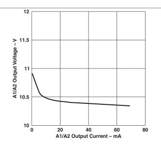
Figure 2. A1/A2 Output Voltage vs A1/A2 Output Current
