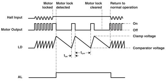
Figure 3. Motor Lock Diagram
