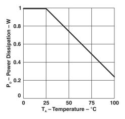
Figure 10. Power Dissipation
