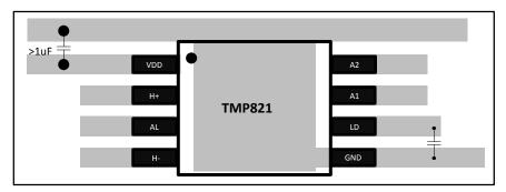
Figure 9. Recommended Layout Example
