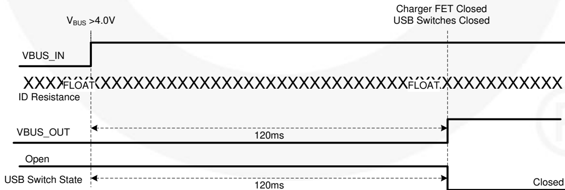
Figure 10. USB Standard Downstream Port Attach Timing (19)
