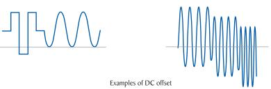
The 9830B Series is capable of generating AC+DC waveforms. When operating in pulse, step and list mode, the AC signal can be combined with either a positive or negative DC offset voltage, allowing users to create a wide range of waveforms.
