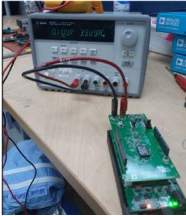
Figure 18. Current Input Test Setup Photo
