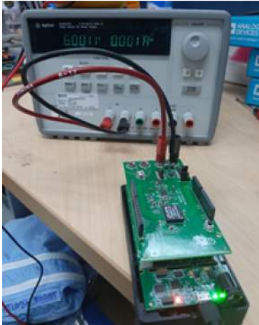
Figure 14. Voltage Input Test Setup Photo
