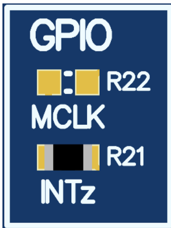
Figure 2-16. GPIO1 Hardware Configuration
