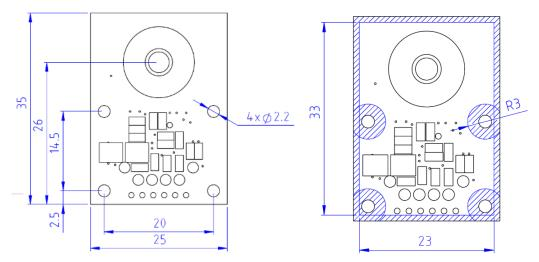
Only use hatched areas for mechanical assembly (screws, nuts, etc).
