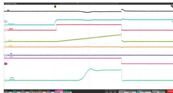
Figure 9-7. Power Up into Short: V_{IN} = 12 V, EN/UVLO Stepped Up From 0 V to 3 V, R_{IREF} = 40.2 k \Omega , R_{ILIM} on Each Device = 300 \Omega , and OUT Shorted to GND
