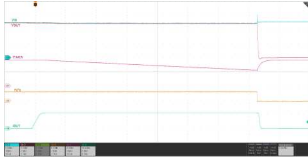
I_{OCP} = 50\text{ A} , t_{TIMER} = 14\text{ ms} , I_{OUT} stays above the I_{OCP} threshold persistently to trigger circuit-breaker response
