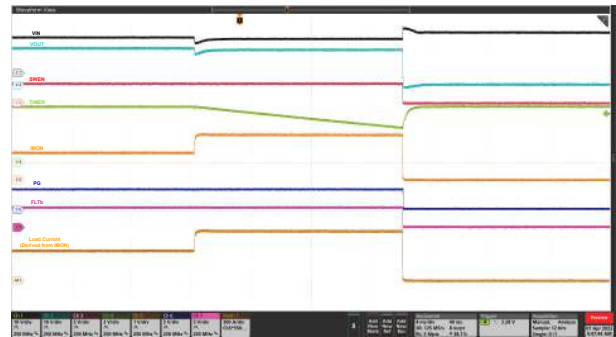
Figure 9-11. Circuit-Breaker Response: V_{IN} = 12\text{ V} , C_{TIMER} = 22\text{ nF} , C_{LOAD} = 55\text{ mF} , R_{IMON} = 167\text{ }\Omega , R_{IREF} = 40.2\text{ k}\Omega , and Load Current Stepped up From 300 A to 500 A for > 20 ms
