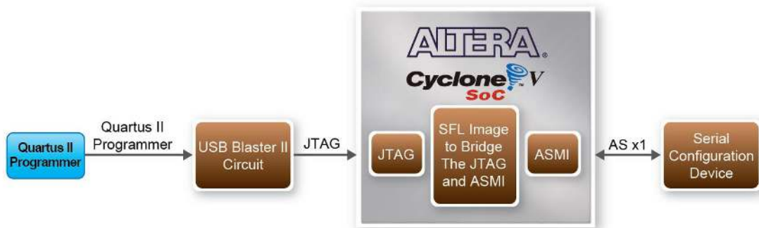
Figure 3-9 Programming a serial configuration device with SFL solution
