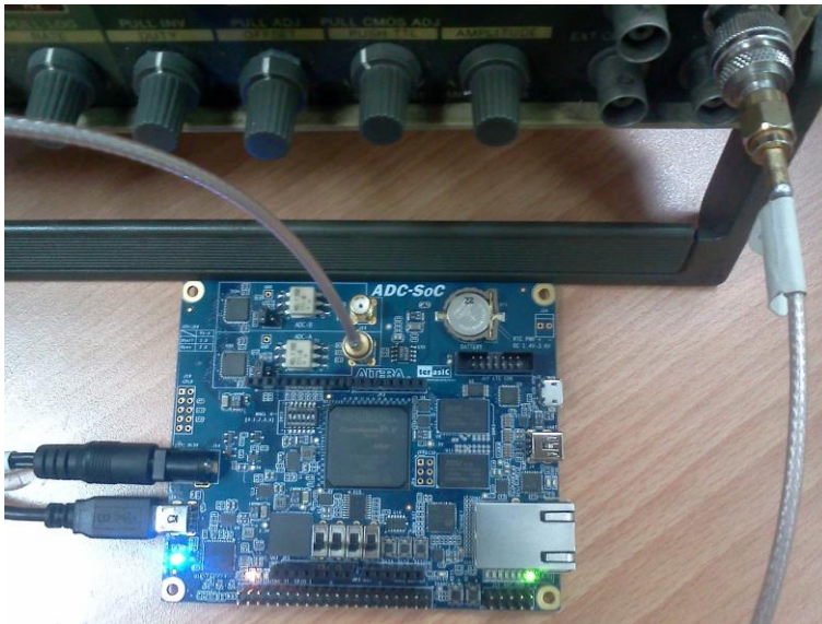
Figure 4-6 Hardware setup for the HIGH-SPEED-ADC
