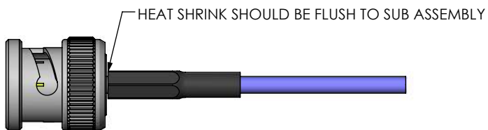
IN-PROCESS 5 ACTIVATE HEAT SHRINK
