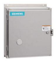
Non-reversing NEMA contactor, Size 2, Three phase full voltage, Contactor amp rating 45A, 3 wire (NO aux included), 208VAC 60Hz coil, Non-combination type, Encl NEMA type 4X 304 S-Steel, Water/dust tight noncorrosive, Extra-wide enclosure
