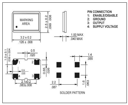
NOTE: A capacitor of 0.01  $\mu\text{F}$  between Vcc and Ground is recommended
