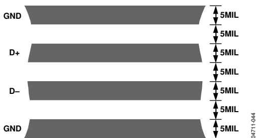
Figure 25. Arrangement of Signal Tracks
