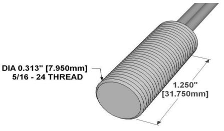
All measurements are in Inches [millimeters]
