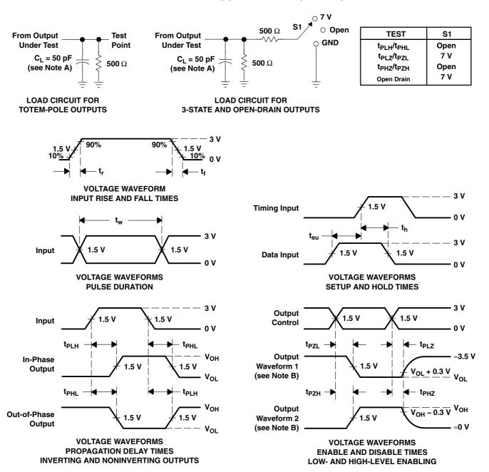
NOTES: A.  $C_L$  includes probe and jig capacitance.
