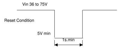
The connection to a RC pin controls an Isolated DC-DC Converter to turn on/off. While the Isolated DC-DC Converter is halted under the remote control, alarm function does not operate; refer to Alarm Output.
