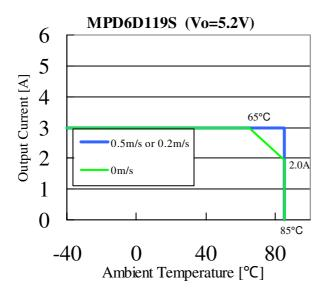
9-1-3-2 .Typical Power derating of MPD6D111S Nominal output currents are attainable in Vin=36 to 60V or Vin=60 to 75V with various air flows of 0.2m/s(40LFM),0.5m/s(100LFM),0.8m/s(160LFM),1.0m/s(200LFM).
