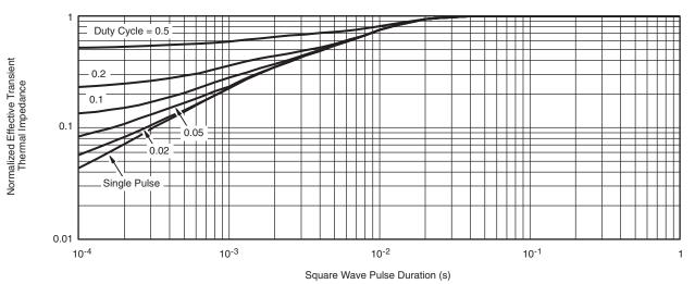
Normalized Thermal Transient Impedance, Junction-to-Case
