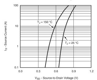
Source-Drain Diode Forward Voltage
