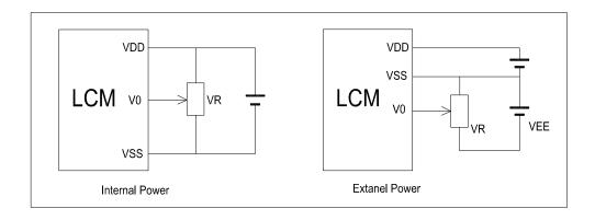
$V_{DD\sim}V_0$ : LCD Driving voltage VR:  $10k\sim20k$
