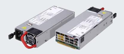
Advanced Energy's Artesyn DS2000SPE is an ultra-high denstiy power supply providing 50W per cubic inch. The 2000 watt DS2000SPE power supply is housed in 1U high rack-mounting enclosures measuring just 3.4 x 7.7 inches (86.3 x 196.5 mm). This form factor is significantly shorter than that of similarly rated earlier-generation power supplies — freeing up valuable system space — and is achieved by use of the latest power switching technology and high density component packaging techniques.
